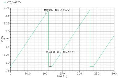
Figure 17 - 12Bit ADC ramp simulation
