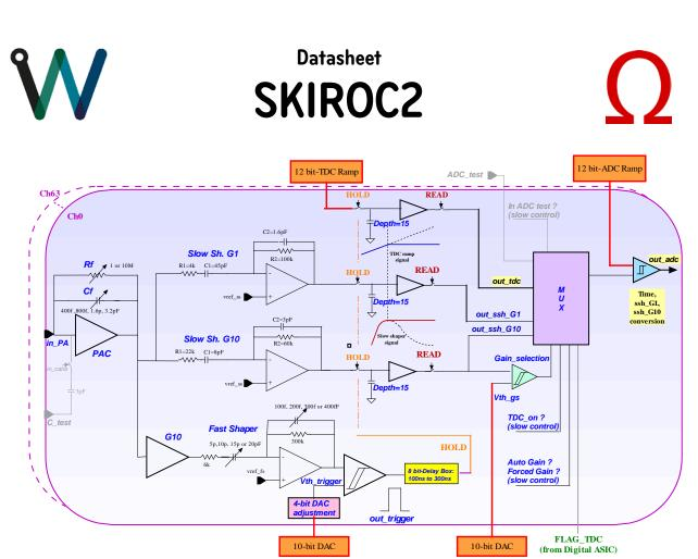
Figure 4 - SKIROC2 : Analog part simplified scheme
