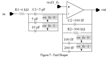
The response for 1 MIP at the input of the PAC (C $\not=$ 6pF) has been simulated.
