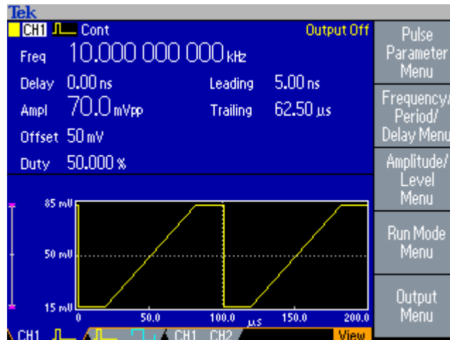
Figure 22 – Pulsar injection signal
