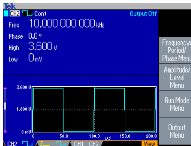
Figure 24 – Synchronisation signal for S-curves test
