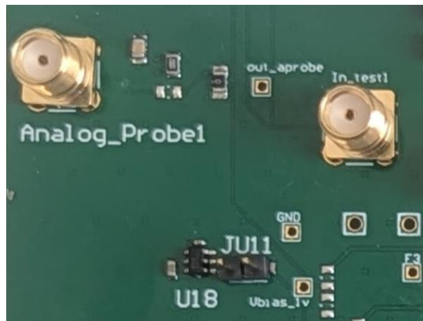
Figure 32 - SMA input injectors and Analog_Probe output (top-left corner of the board).
