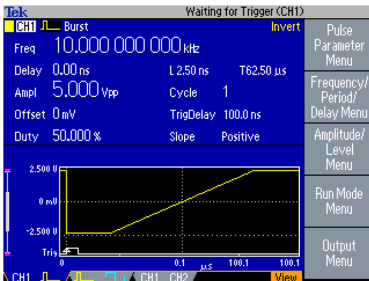
Figure 22 – Pulser injection signal
